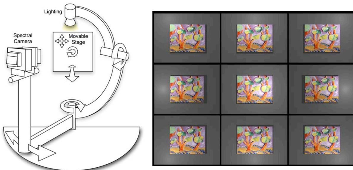
Figure 6. Imaging goni-spectrophotometer instrument used to capture BRDF of artwork (Left) and sample image sequence (right) for one sweep of the light source at a fixed camera position.
