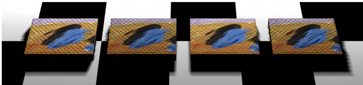
*Figure 5. Renderings of painting surface using, from left to right, anisotropic, Blinn, Lambertian, and Phong BRDF algorithms.*
