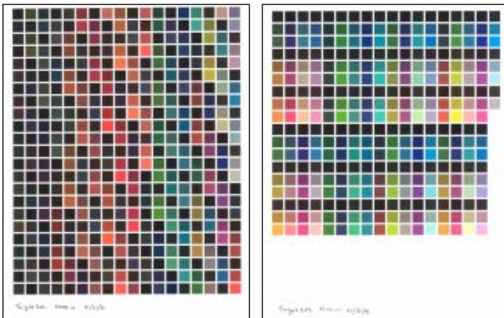
**Figure 4-4 - Targets displaying 729 Neugebauer primaries of Cellular YNSN model.**
