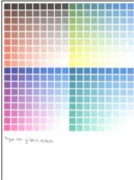
**Figure 3-5 - Four of the fifteen two color overprint grid targets.**
