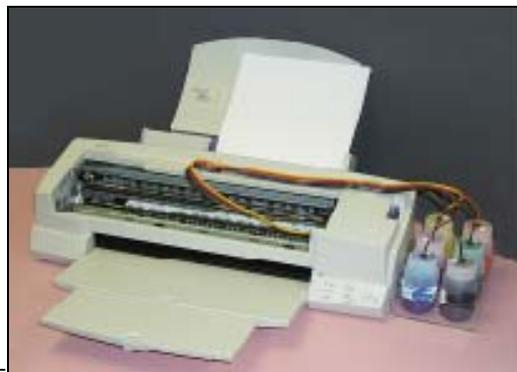
**Figure 2-1 - Modified Epson Stylus Photo 1200 printer with CYMKOG inkset and continuous-feed system.**
