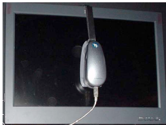
Figure 12. IBM T221 monitor and Eye-One setup for the experiment.
