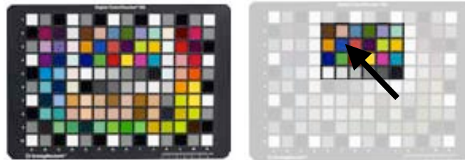
Figure 3(a). (Left) Color Checker Digital SG target; (b). (Right) Traditional 24-patch target found within SG, used to build the camera ICC profile.
